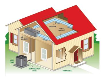
**Emergency Heating:** Should the heat pump fail, activate the emergency switch on the thermo-stat. The red light indicates that it is on. This will stop the heat pump from operating and will provide supplemental heat until the HVAC contractor arrives.
